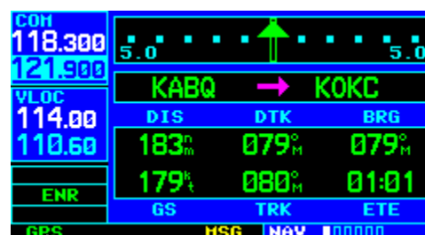
Figure 9-9 GPS Coupled to External CDI
